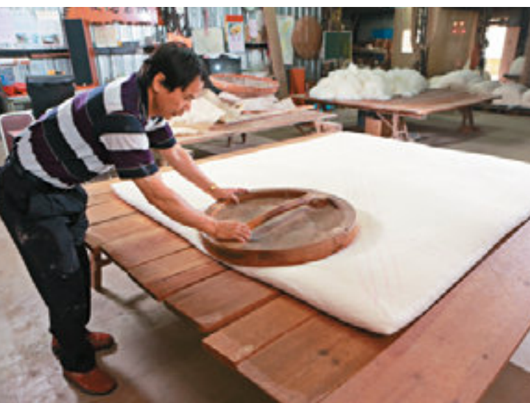
It takes skill to use a tool to twist cotton fibers. If it's perfectly done, the remaining steps are easier for the comforter maker.
